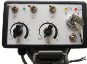
The ELSK 106-15\*\*\* unit is used to control a proportional solenoid. It consists of the ESSK 106-91\*\*\* module, fitted in a aluminium housing. The housing is provided with a front plate with an ON/OFF-switch, a green LED and a control signal potentiometer with indicator knob.
